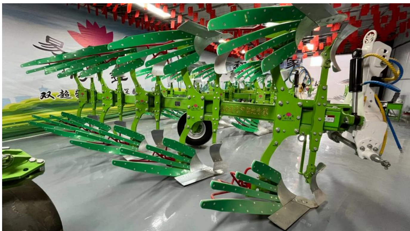
1LYFT-550 Type Side-shift Hydraulic Reversible Plow
