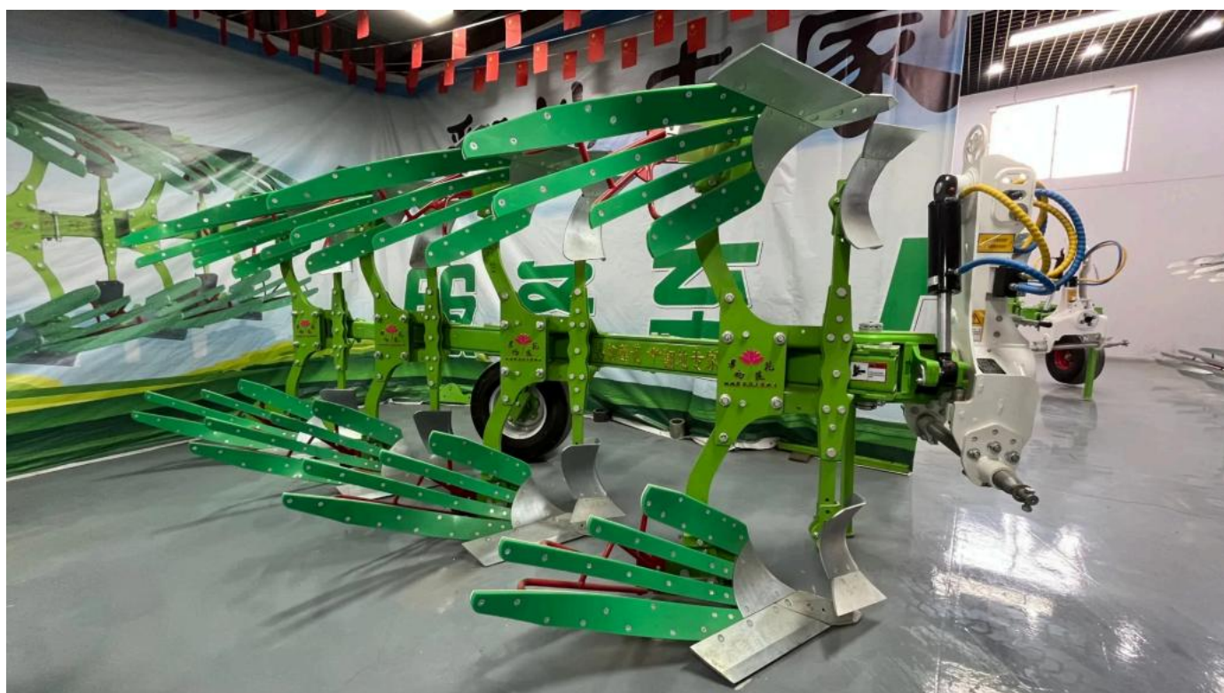
1LYFT-450 Type Single Lead Screw Hydraulic Reversible Plow
