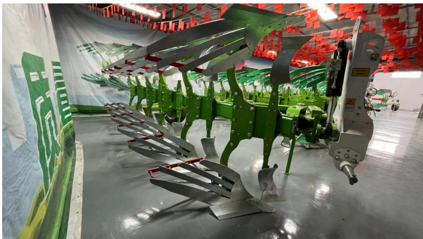
1LYFT-650 Type Side-shift Hydraulic Reversible Plow
