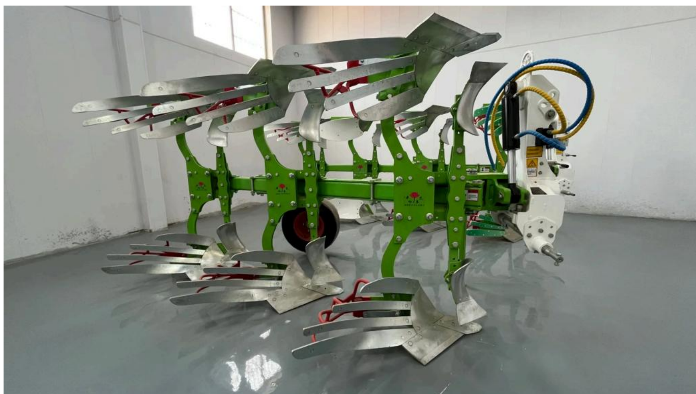
1LYFT-340 Type Single Lead Screw Hydraulic Reversible Plow
