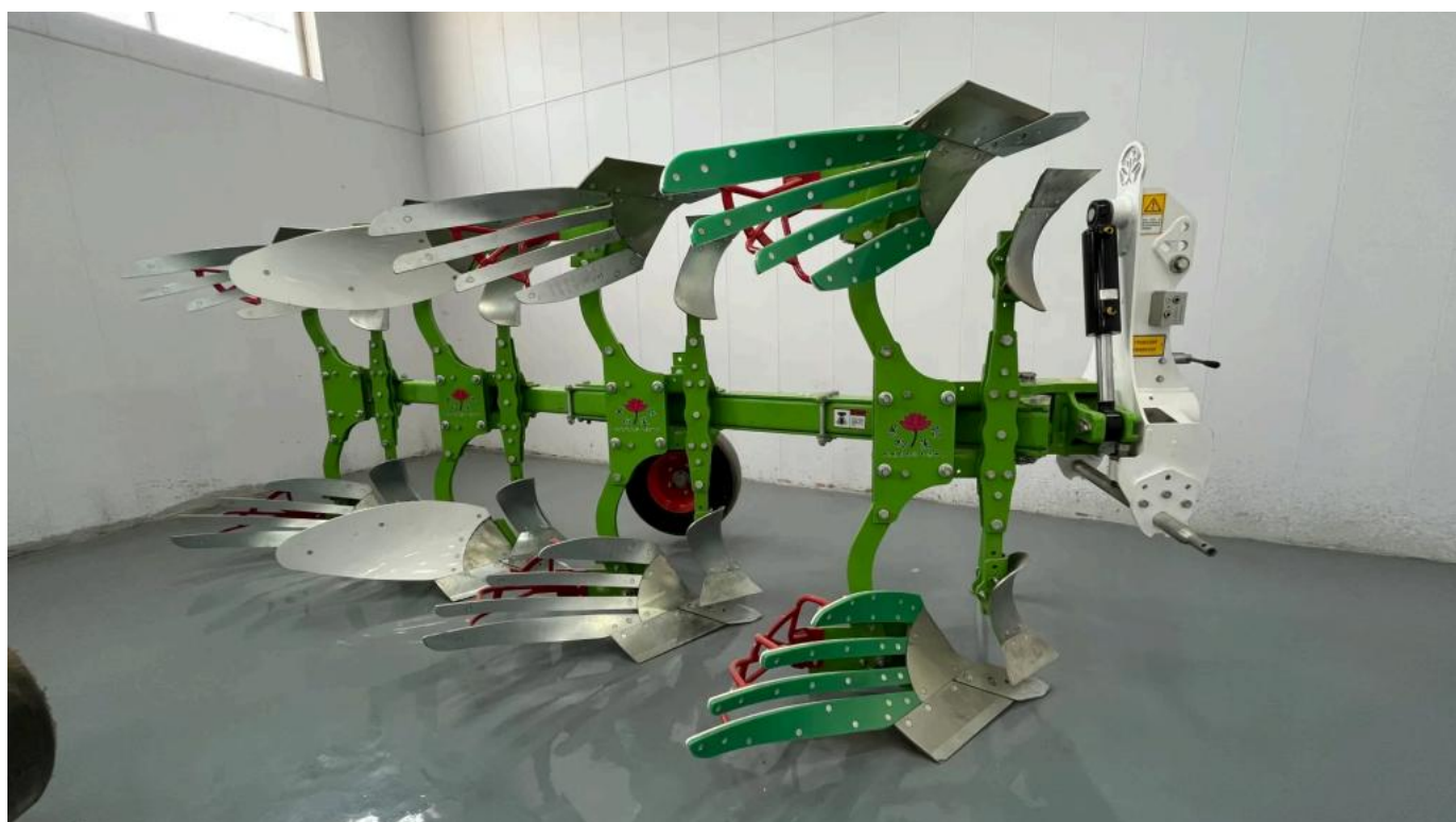
1LYFT-440 Type Single Lead Screw Hydraulic Reversible Plow
