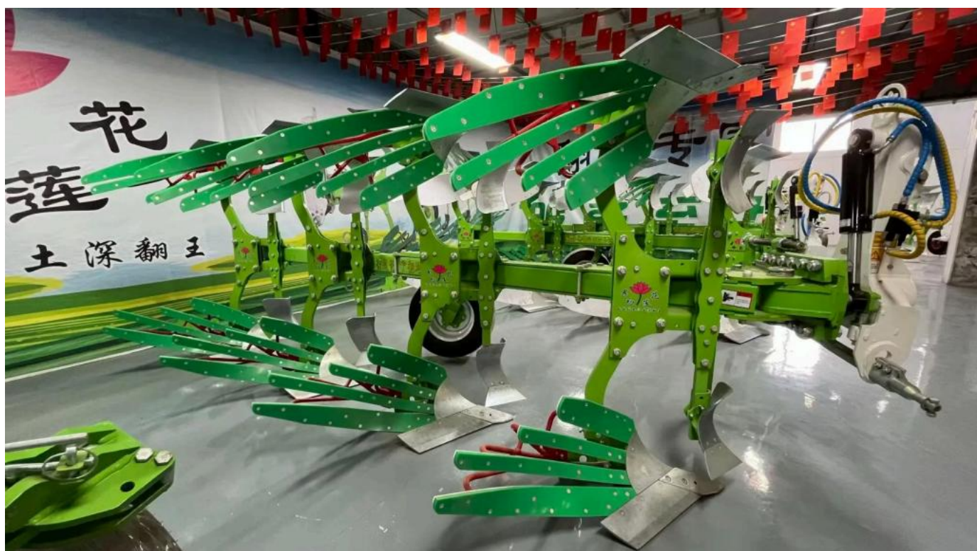
1LYFT-450 Type Side-shift Hydraulic Reversible Plow
