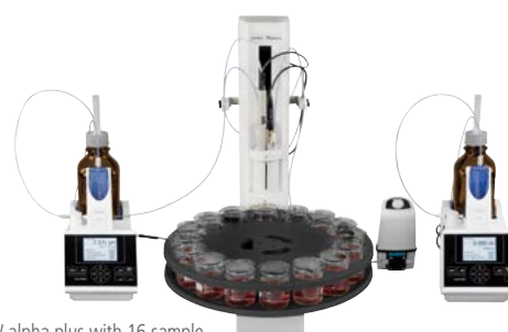
TW alpha plus with 16 sample dish and pump MP 25
